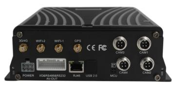
The **JH4-HD** is a **AHD 4 channel Mobile DVR** designed for on-board vehicle recording. It has four ports to record up to four cameras simultaneously and an ethernet port to connect a forward-facing IP camera. The system comes with GPS to record the vehicle location and driving route as well. Footage records onto an included 4TB hard disk with backup recording (256GB) onto 1 SD card.
