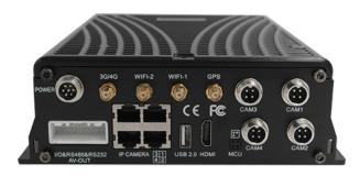
JH4-HYBRID is a Mobile NVR designed for on-board vehicle recording which comes with remote live video viewing. This system is able to to connect to a WiFi hotspot in your vehicle. This model is compatible with jetpacks from all major carriers. Perfect for fleet tracking (can be used as a GPS tracker) and fleet management this NVR allows you to easily view and download footage even while the vehicle is on the road!
