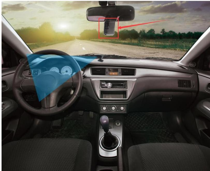
Figure 5. ADAS camera installed in the windshield of a small car
